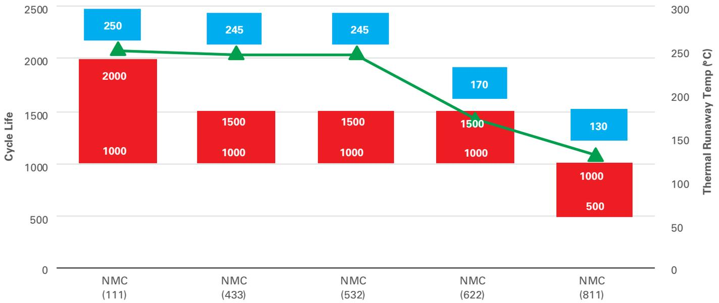
Source: Bloomberg New Energy Finance. Nickel-manganese-cobalt (NMC) cathodes with different ratios of each material. For example, NMC (111) contains equal parts nickel, manganese and cobalt.
